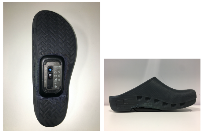
Fig. 4. Mouse clog. We can observe the wireless mouse does not interfere with the clog form factor.
