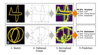
Figure 7: Sketch recognition process: the 3D strokes are first projected onto a 2D best-fitting plane to get a flattened image. Flattened images are then converted to normalized bitmaps. The recognition model offers a list of predictions with confidence based on the bitmaps. Sketch A is an airplane, and Sketch B is a basketball.
