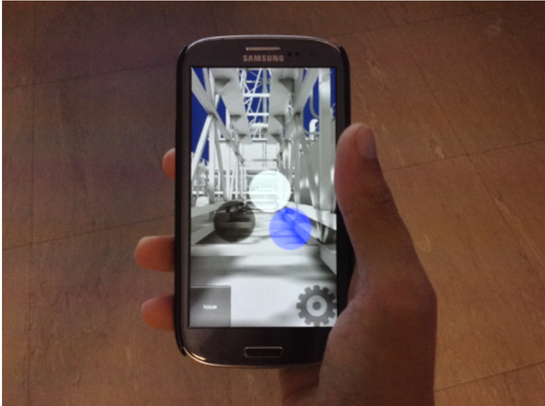
Figure 3.13: GUI approach to associate people with their devices. The dark circle represents a traced user that is yet to be associated with a device. The blue circle is a currently authenticated user and the white one is a authenticated user from a remote location.
