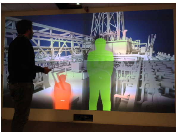
Figure 3.6: Users' shadows depicting two participants on the wall display. The larger shadow indicates that the remote person had the moderator role (in green). Local participants (on the left) also have a shadow representation.
