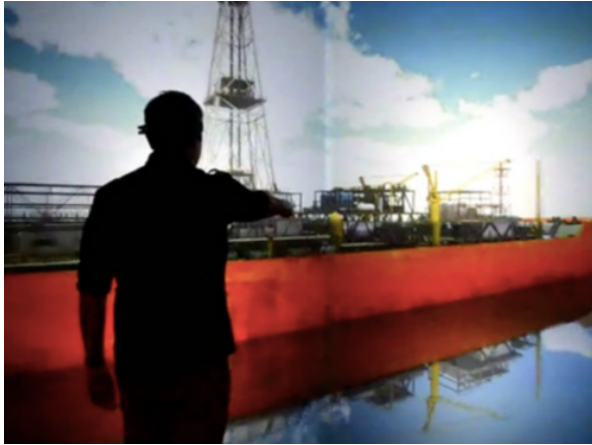
Figure 3.14: Navigation using a Brain Computer Interface. Pointing gestures combined with electroencephalographic data results in a forward movement of the virtual environment's camera to the point of interest
