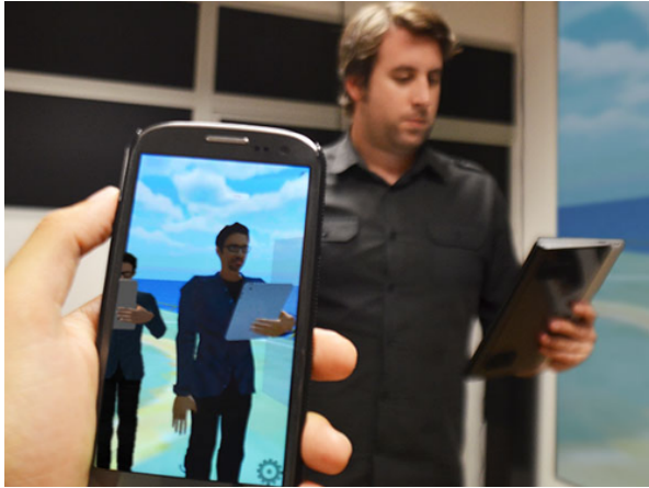
Figure 3.8: Virtual window offers a personal view to the virtual world, showing users' avatars with their position and orientation accordingly to the wall, from the device owner's point of view. In this case two users are shown, one local and one remote.
