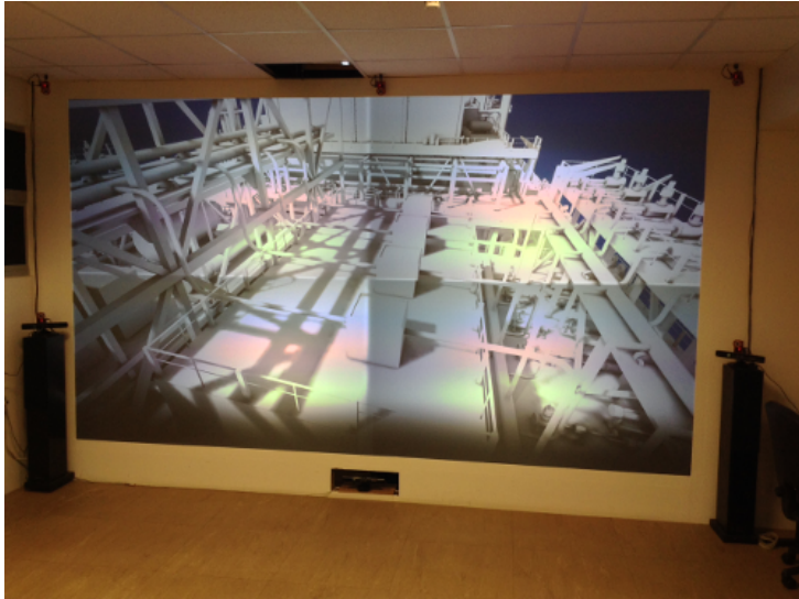
Figure 4.12: Main Setup, comprised of a large scale display, Kinect depth cameras and a ceiling-mounted projector
