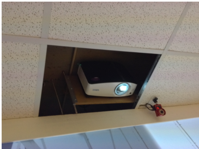
Figure 4.14: Ceiling-Mounted Projector, installed above the wall display to display the floor shadows awareness technique.
