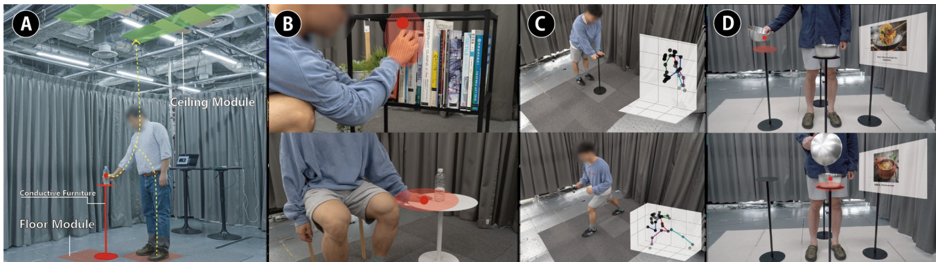
Figure 1: CapAura turns an ordinary floor carpet and everyday conductive furniture into a room-scale capacitive sensing field. (A) Electrodes integrated into the floor modules and ceiling modules, with conductive furniture acting as passive electric field extenders, enable room-scale proxemic sensing. (B) When a user touches or hovers near a surface, our system senses this interaction. (C) The system jointly detects Position, Identity, Movement, and Orientation (PIMO) without cameras or worn devices. (D) Detected proxemic events drive spatial hotkey interactions, turning the living space into an ambient spatial interface.
